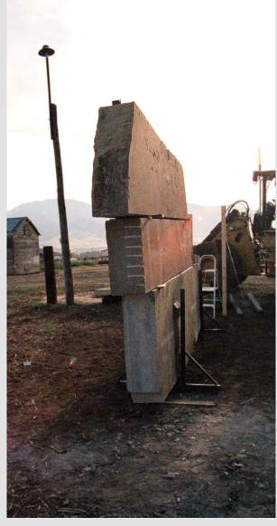
25 tons of very strong durable stone is classified a sedimentary rock but composed of fine sand and clays, compressed to an exquisite hardness that allows it to be polished to a steely sheen. The only sedimentary stone I know of that can do that.
